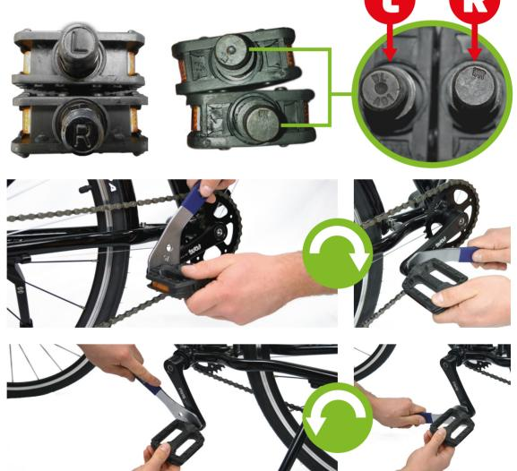
Non Drive-side: hold the "L" pedal & turn the threaded shaft Anti-Clockwise to tighten.
