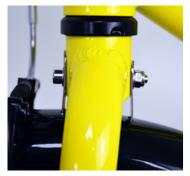
2. Insert the bolt with a metal washer on either side of the adjustable bracket, and lightly tighten the nut.
