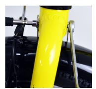
5. Tighten up the mudguard to secure it with the spanner and allen key to 4Nm.
