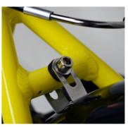
7. Tighten up the mudguard to secure it with the spanner and allen key to 4Nm.
