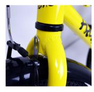
1. Place the mudguard between the fork legs, ensure that one metal tab is placed in front of the fork and one metal tab behind the fork.
