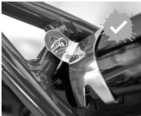
How the bracket should sit above the seat stays
