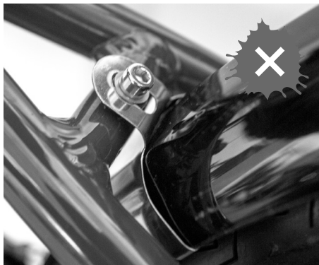
Do not mount the bracket in between the seat stays
